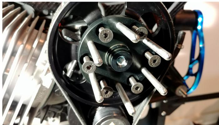
4. Using the long end of a 4mm Allen Key lightly tighten the six bolts in a crisscross pattern.
