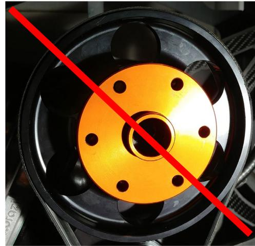
2. Remove the Cam Lock/Prop Plate assembly from the Quick Release Hub and place the main Hub (with pins) onto the upper reduction pulley lining up the bolt holes.
