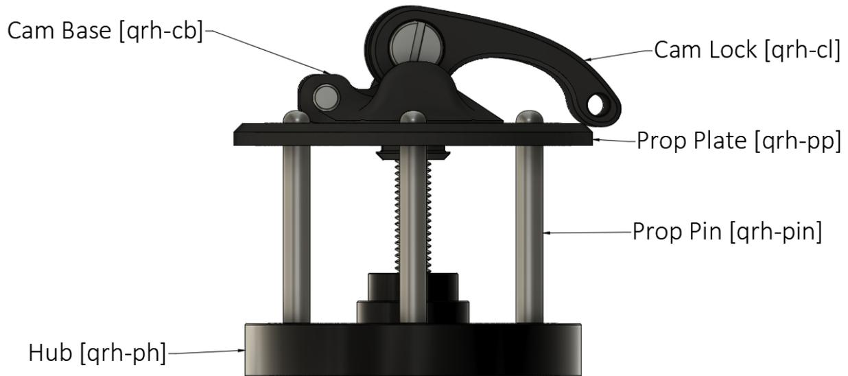
**Cam Base [qrh-cb]:** Nylon Cam Base with Counter-Balance pin. This part is replaced as an assembly (including pin) and it snaps into the Prop Plate without hardware.
